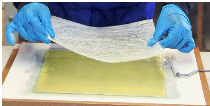
Figure 2. Roll the glass cloth together with the resin and hardener; the compound results in a new material – fiberglass ( Molding materials . https://www.23stroi.ru/catalog/poliehfirnye_smoly/valiki-prikatochnye-v-assortimente/ )
